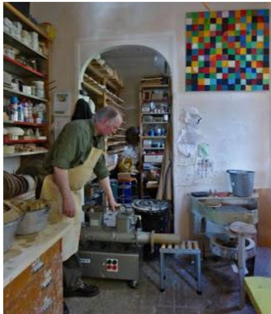
Ha, Ha... the pugmill is a delight to use. There is a steady rumble of motor and vacuum pump, but not unpleasantly so, and I can still listen to the radio and operate the machine at the same time. On first use I processed about 40kg of scrap clay in about 15 minutes (the pugmill is rated to do 200kg per hour). I immediately made a vase from the freshly pugged clay, which I found to be very even in texture, airless, and very good to throw.
