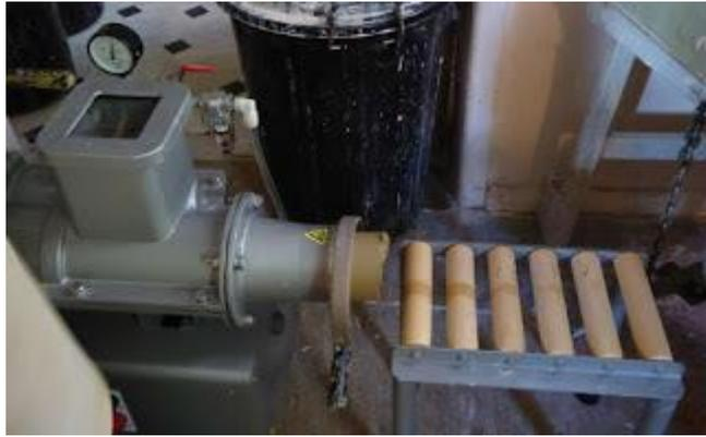
In spite of all the dire safety warnings in the manual, the machine is very safe to use as the augers only turn after clay has been put in and the lid shut. When the lid is opened, the augers are stationary, which means the chances of hands being chopped up by whirling blades is minimal.
